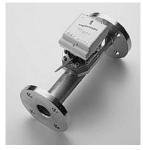
The independent flow sensor, which is combinable with any integrator. The flow is converted into pulses, which are transmitted to a integrator where they are counted and used to calculate flow and energy consumption.
